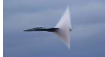
Fig.13 Sonic boom pressure condensates the water vapor in shape of Mach cone.
