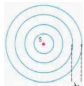
Fig.6 "λ" for a source at rest emitting spherical wave fronts.
